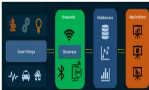
Figure 1. IoT communication architecture
