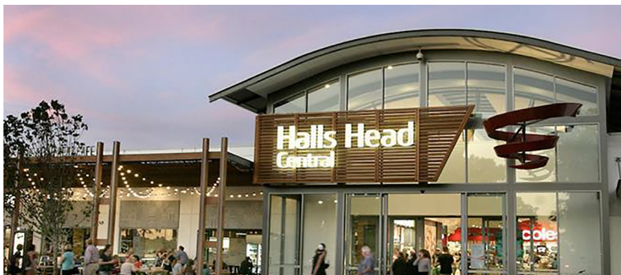
The ribbon consists of Divinycell Matrix IPN foam core from Diab with stitched E-glass skins using a vinylester resin.
