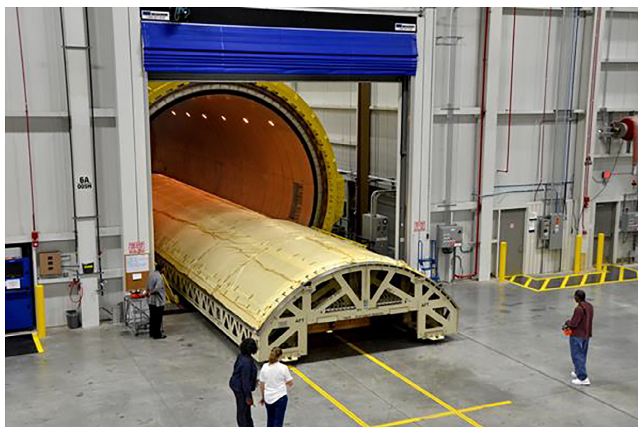
Spirit AeroSystems says that some of the world's largest autoclaves to support the company's composite fuselage business.
