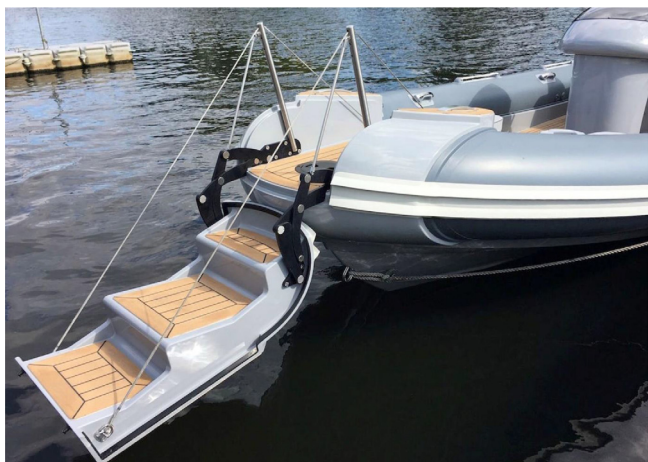
One project incorporated custom concealed hinges for a beach lander bow option.
