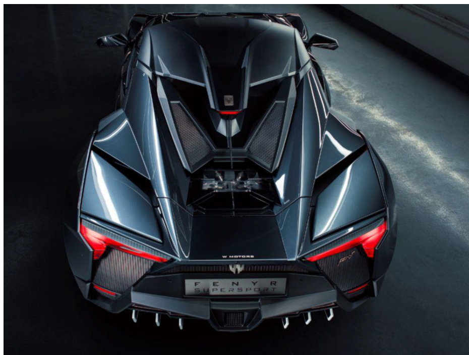
The company developed graphene prepreg to make the W Motors Fenyr SuperSport tailgate.
