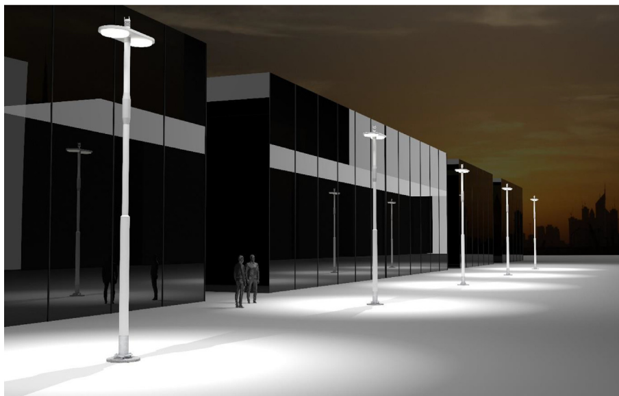
The composite pole functions as mast, architectural casing, weather protection and radome for the 5G antenna.
