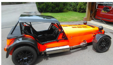
A lightweight CRFP roof custom designed using Scott Bader Crestapol 1260 resin.
