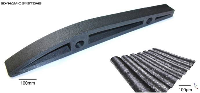
FIGURE 2 A 3D printed nanocomposite full size aircraft wing rib produced to test the dimensional accuracy and a 3D scan showing the layer resolution of the structure with 1% MWCNT.
