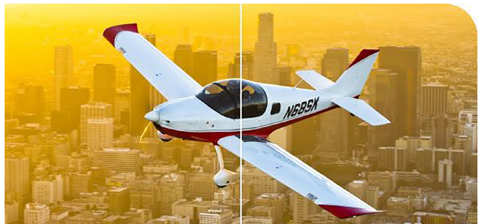
The Sling is a lightweight aluminum and composite aircraft.
