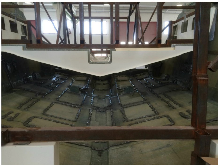
Mastikol used Scigrip's Lloyd's approved SG230 HVA adhesive, supplied in 189 litre drums.
