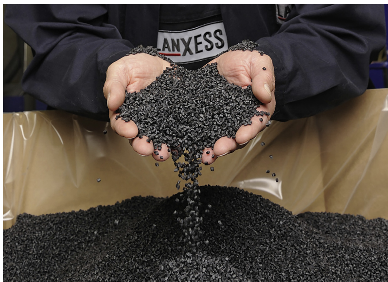
Durethan engineering plastics (PA 6 and PA 6.6 compounds) are used in numerous applications. (Photo courtesy Lanxess AG.)
