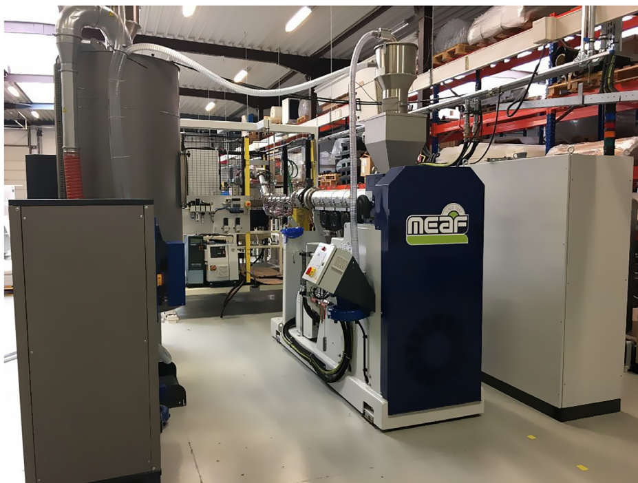
EconCore partnered with MEAF to develop lab extruder for continuous thermoplastic honeycomb production.
