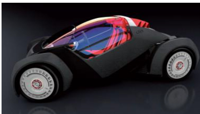
A carbon fiber reinforced thermoplastic compound from chemicals company Sabic was used to produce the world's first 3D-printed vehicle.
